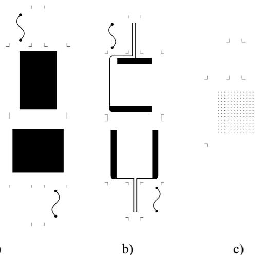
Fig.4. a) ITO pattern , b) Ag electrodes and c) insulating layer
