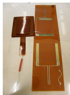
Fig.6. Printing touch screen onto flexible substrate
