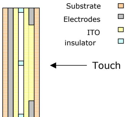
Fig.5. Schematic of the touch screen
